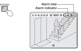
If consecutive alarms are detected on the same channel, depending on the alarm retrigger setting, they may be counted as one alarm. (P60)
